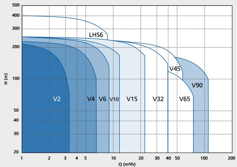
**Movitec characteristic curves 60 Hz, 3500 1/min**
